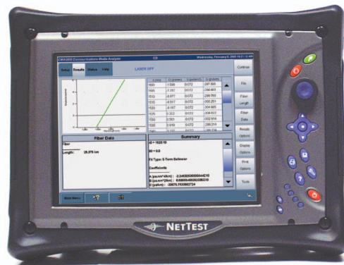
The OTDR/CD module is an advanced solution for measuring chromatic dispersion and loss in one module.
